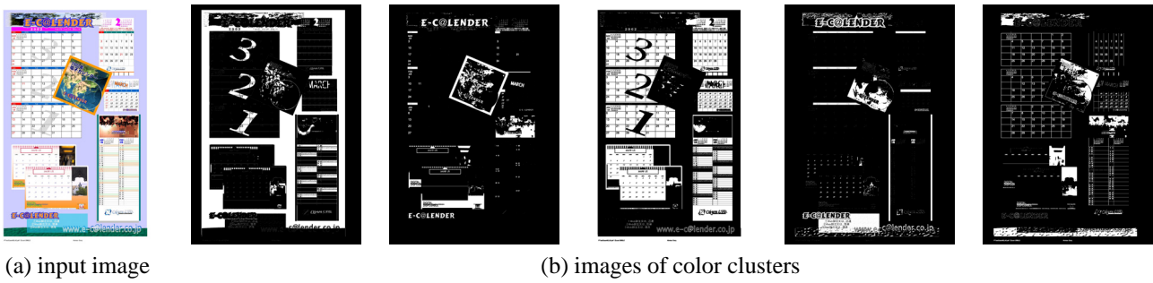
Figure 2. An image is decomposed into k images of color clusters. ( k = 5 )
