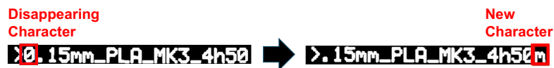
Fig. 6. Text horizontally scrolls if the length of the text exceeds 19 characters. In the scroll, the leftmost character disappears, and a new character appears on the right.
