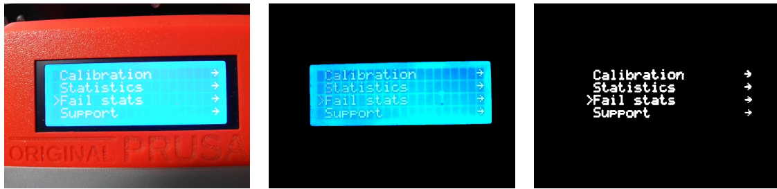
(a) The average image of the last ten display snapshots. (b) Display area with white text and a blue background. (c) Binarized text regions.
