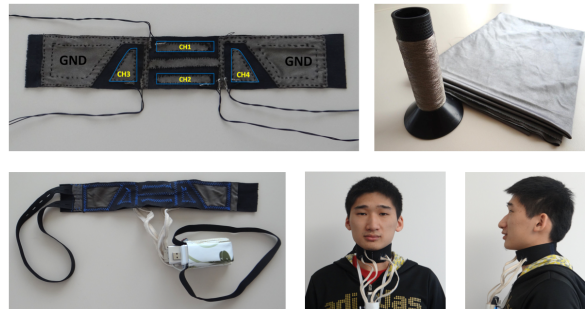
Figure 1: The material, the sensor pad design and the ready neckband worn by a test subject
