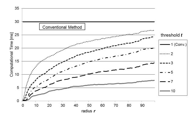
Figure 4.3 The computational time in character recognition process except feature extraction and matching.
