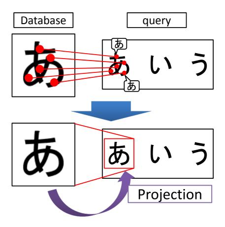
Figure 2.2 A detail of the character recognition process.
