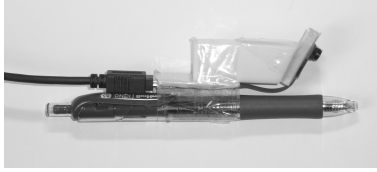
Figure 3. The camera pen, containing an ordinary ballpoint pen and a tiny USB camera.
